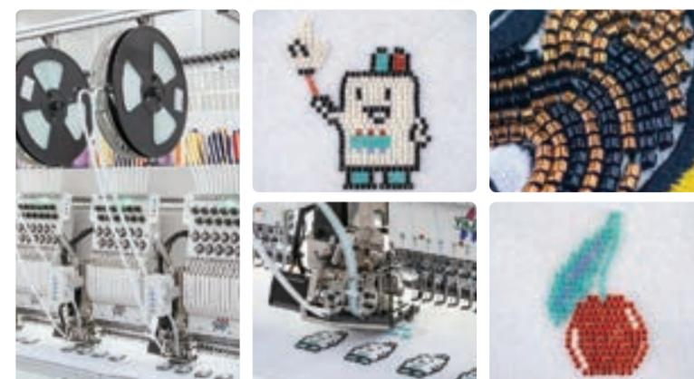
Automatic Color Change Glass Bead embroidery device. It is automated allowing you to embroider beads rapidly instead of by hand so that mass production becomes possible. Also, the beads are set in a tape reel so it is easy to exchange and manage.
